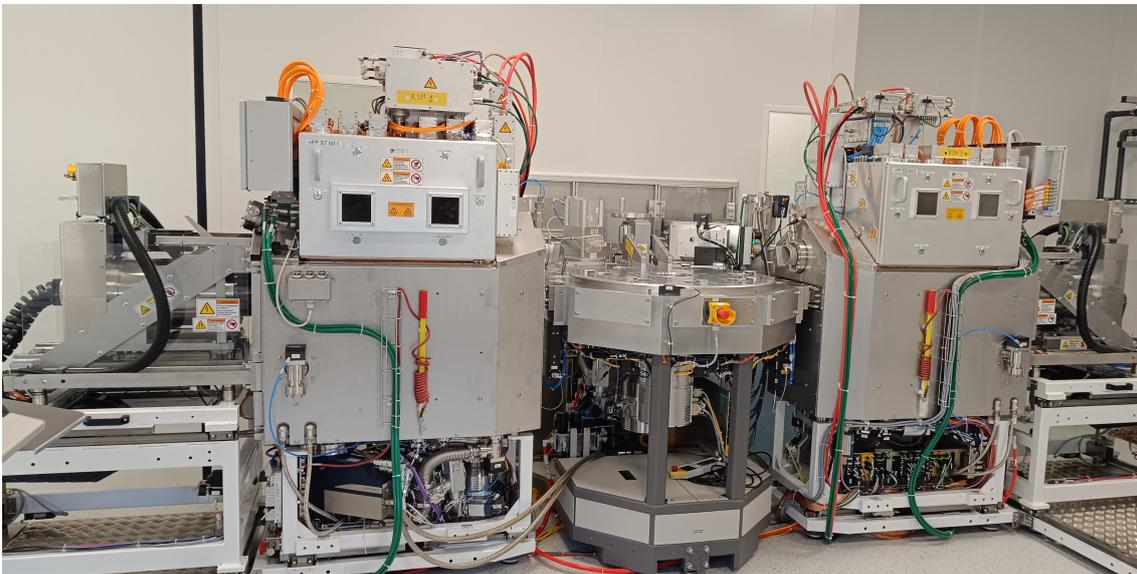
Figure 1: The Singulus tool with two modules (left and right) and the transfer chamber (center) installed at Spintec.
